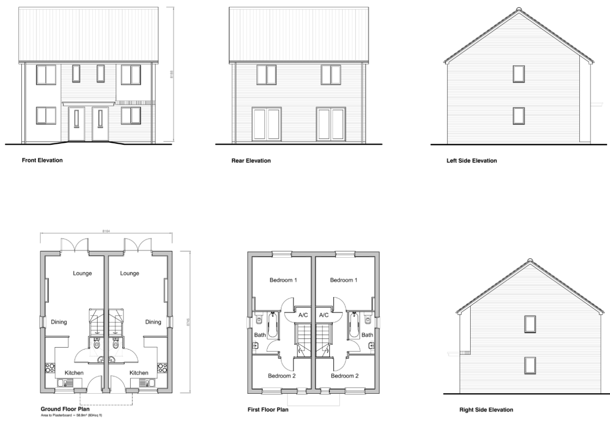
Type 3N Floor Plans & Elevations Plots 63, 64, 67, 68 Area to Plasterboard = 58.9m 2 (634sq ft)
